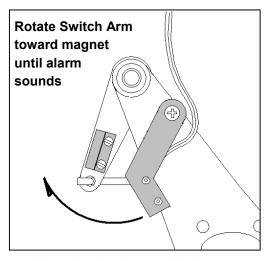
Hold switch arm firmly in position with right hand and tighten lock-nut in this position using hex key provided.
